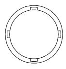
© HOLE IN CHASSIS: Ø2.845 ◎ CHASSIS THICKNESS: 1.0 mm
