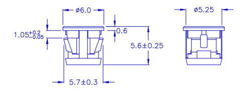
© HOLE IN CHASSIS: Ø5.3+0.05
