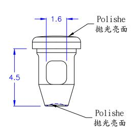
⊚ HOLE IN CHASSIS: Ø3.2 mm © CHASSIS THICKNESS: 0.8 mm
