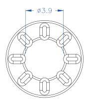
$\odot$  HOLE IN CHASSIS:  $\emptyset 5.5^{+0.05}_{-0}$  mm  $\odot$  CHASSIS THICKNESS:  $0.8^{+0}_{-0.05}$  mm
