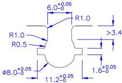
$\bigcirc$  CHASSIS THICKNESS: 1.0 $^{+0}_{-0.05}$  mm
