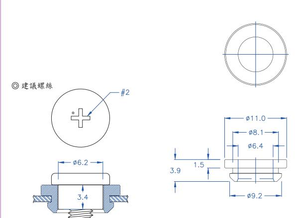
$\bigcirc$  HOLE IN CHASSIS:  $\emptyset 8.1^{+0.05}_{-0}$  mm
