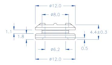
$\odot$  HOLE IN CHASSIS:  $\emptyset 8.2^{+0.05}_{-0}$  mm  $\odot$  CHASSIS THICKNESS:  $1.0^{+0}_{-0.05}$  mm
