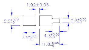
$\bigcirc$  CHASSIS THICKNESS: 0.8 $^{+0}_{-0.05}$  mm
