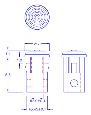
O HOLE IN CHASSIS: Ø3.5
