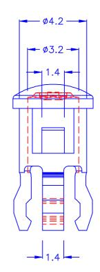
◎ HOLE IN CHASSIS: Ø4.3 mm ◎ CHASSIS THICKNESS: 1.1 mm
