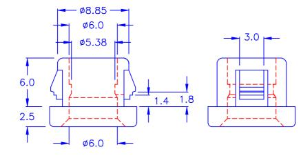
© CHASSIS THICKNESS: 1.2∼1.6 mm © HOLE IN CHASSIS:
