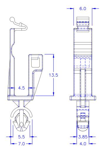
O HOLE IN CHASSIS: Ø4.0
