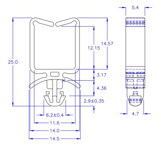
O HOLE IN CHASSIS: Ø4.8
