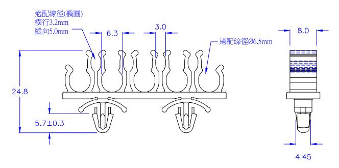
O HOLE IN CHASSIS: Ø4.6
