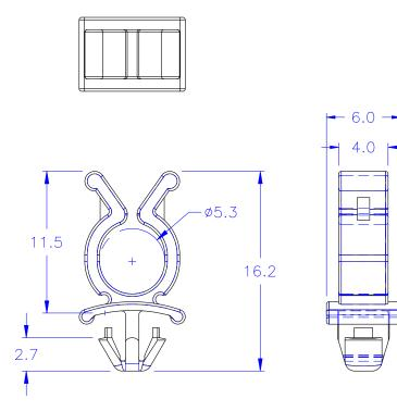
$\odot$  HOLE IN CHASSIS:  $\emptyset 4.3^{+0.05}_{-0.05}$  mm  $\odot$  CHASSIS THICKNESS:  $1.6^{+0}_{-0.05}$  mm
