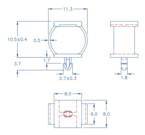
O HOLE IN CHASSIS: Ø2.0
