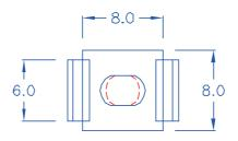
© HOLE IN P.C.B: Ø3.5 mm © P.C.B THICKNESS: 1.2 mm
