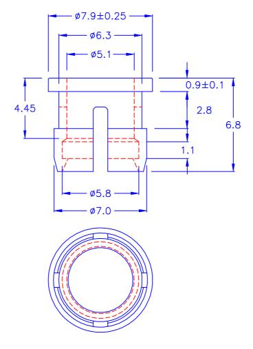
© HOLE IN CHASSIS: Ø6.4
