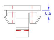
O HOLE IN CHASSIS: Ø5.0
