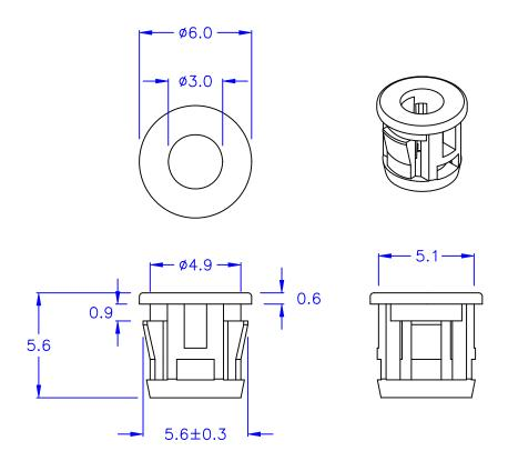
© CHASSIS THICKNESS: 0.8 mm © HOLE IN CHASSIS: Ø5.2 ±8.1
