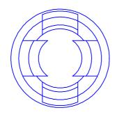
OHOLE IN CHASSIS: Ø4.3 mm
