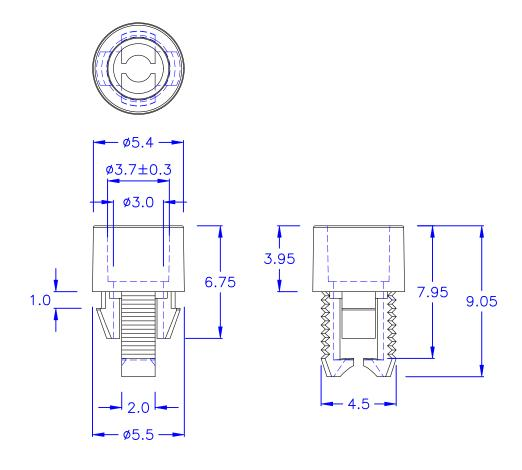
O HOLE IN CHASSIS: Ø4.5
