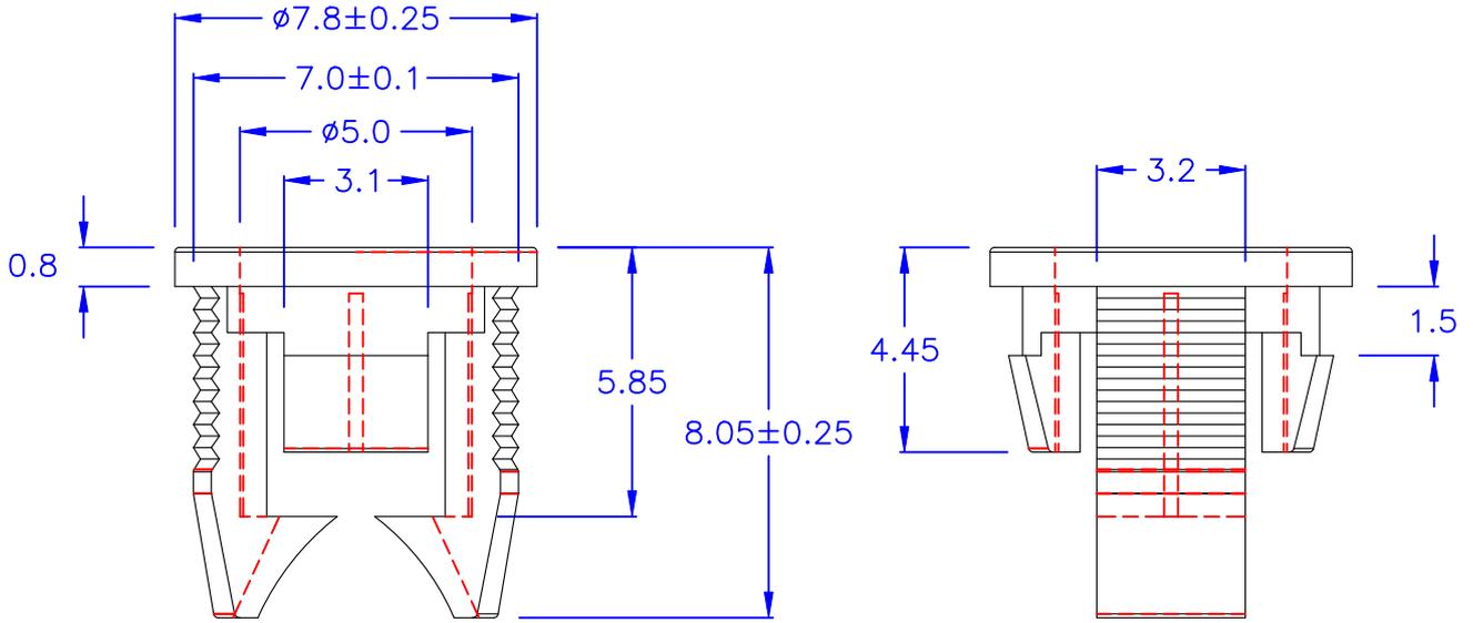
◎ HOLE IN P.C.B.:  $\phi 6.5 \sim \phi 6.6$
