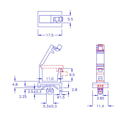
$\bigcirc$  CHASSIS THICKNESS: 0.8~1.0 mm  $\bigcirc$  HOLE IN CHASSIS :
