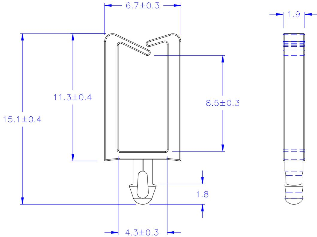
◎ HOLE IN CHASSIS:  $\phi 1.8_{-0}^{+0.05}$  mm
