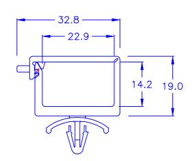
◎ HOLE IN CHASSIS: Ø5.0 mm
