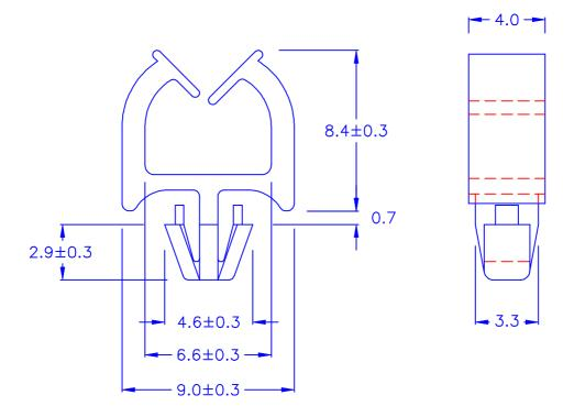
O HOLE IN CHASSIS: Ø3.5
