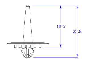
O HOLE IN CHASSIS: Ø4.6
