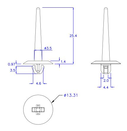
O HOLE IN CHASSIS: Ø4.5
