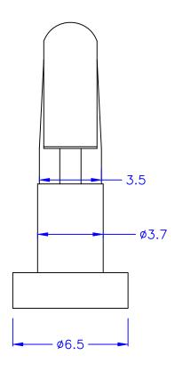
© HOLE IN CHASSIS: Ø4.0
