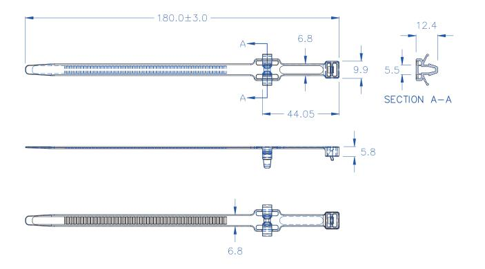
O HOLE IN CHASSIS: Ø5.5±0.1
