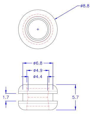
© HOLE IN P.C.B. : Ø6.8mm © P.C.B THICKNESS: 1.6 mm
