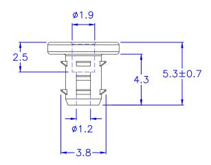
© HOLE IN FAN : Ø3.5mm
