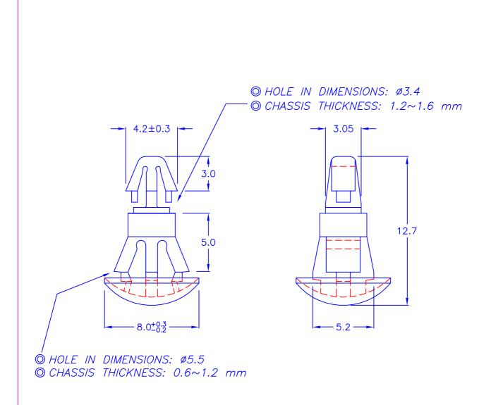
DRAW NO. PGAS016837 PLASTIC TOLERANCE: 網頁圖示供參考,最終以品固公司正式圖面為主 L≤10  $\pm 0.2$ The plastic tolerance is just for your reference; all 10<L≤30  $\pm 0.3$ the measurements and dimensions are according 30<L≤50 ±0.5 to the "DATA SHEET" issued by PINGOOD. 50<L≤100 ±0.7 PART NAME: MATERIAL: N66 V2 or EQUIVALENT 100<L≤250 ±1.2
