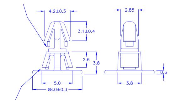
© HOLE IN DIMENSIONS: Ø4.0 © CHASSIS THICKNESS: 0.5mm
