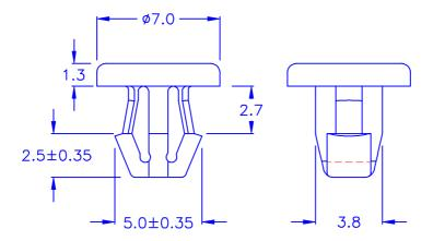
◎ HOLE IN CHASSIS: Ø4.0
