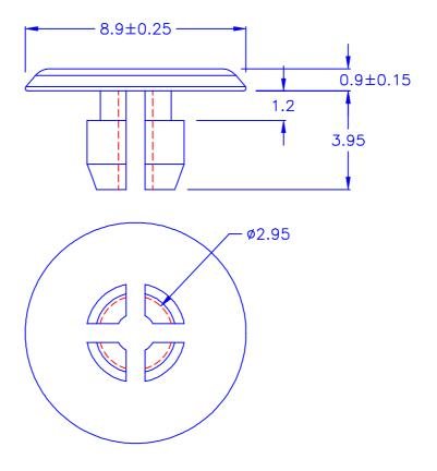
© HOLE IN CHASSIS: Ø3.0
