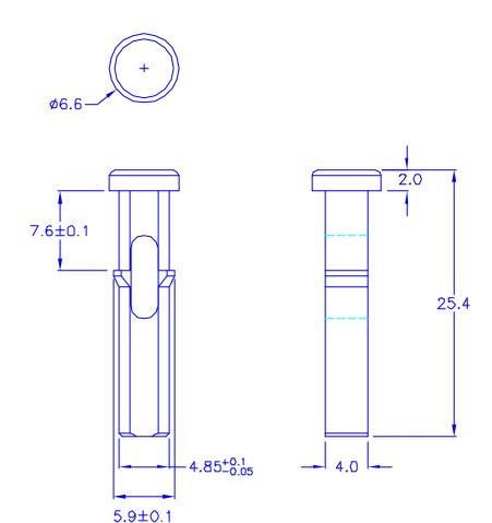
© CHASSIS THICKNESS: 7.0 mm © HOLE IN DIMENSIONS: Ø5.2
