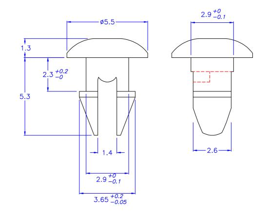
◎ HOLE IN CHASSIS: Ø3.0 ◎ CHASSIS THICKNESS: 2.2 mm
