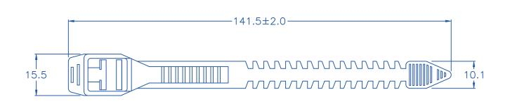
PLASTIC TOLERANCE: 網頁圖示供參考, 最終以品固公司正式圖面為主 ±0.2 L≤10 The plastic tolerance is just for your reference; all 10<L≤30  $\pm 0.3$ the measurements and dimensions are according 30<L≤50  $\pm 0.5$ to the "DATA SHEET" issued by PINGOOD. 50<L≤100 ±0.7 MATERIAL: PE 100<L≤250 ±1.2 COLOR: NATURAL ABOVE 250  $\pm 1.5$ BUNDLE DIA: Ø16 ~ Ø34 SCALE UNIT mm
