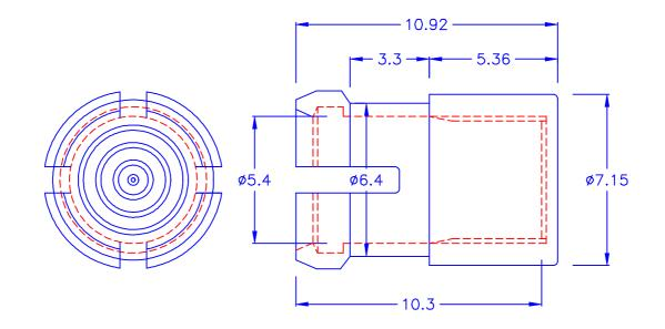
© HOLE IN CHASSIS: Ø6.4 ◎ CHASSIS THICKNESS: 3.2 mm
