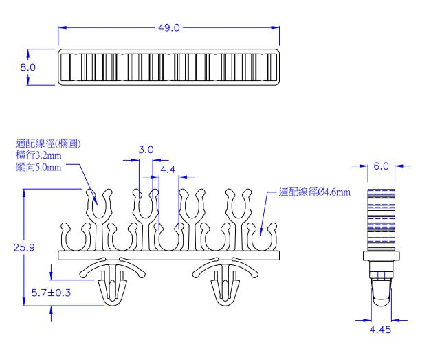
◎ HOLE IN CHASSIS: Ø4.6 ◎ CHASSIS THICKNESS: 0.8~2.0 mm
