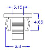
$\bigcirc$  HOLE IN CHASSIS:  $\emptyset 6.3$  CHASSIS THICKNESS:  $0.8 \sim 1.0$  mm  $\bigcirc$  HOLE IN CHASSIS:  $\emptyset 6.5$  CHASSIS THICKNESS:  $1.2 \sim 1.5$  mm
