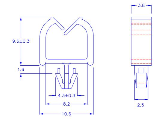
© HOLE IN CHASSIS: Ø2.75 ◎ CHASSIS THICKNESS: 1.4~1.6 mm
