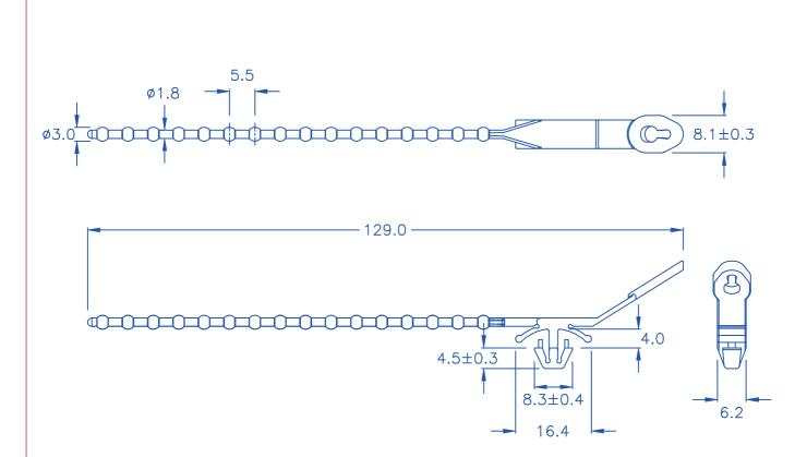
○ HOLE IN CHASSIS: Ø6.5 mm
